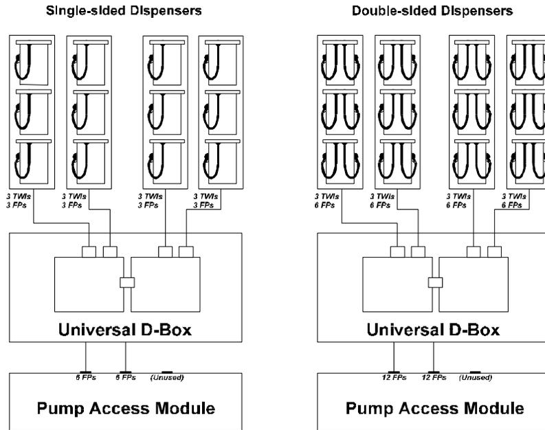
The diagram below illustrates the hardware configuration for 1-12 fueling points with CRIND.
