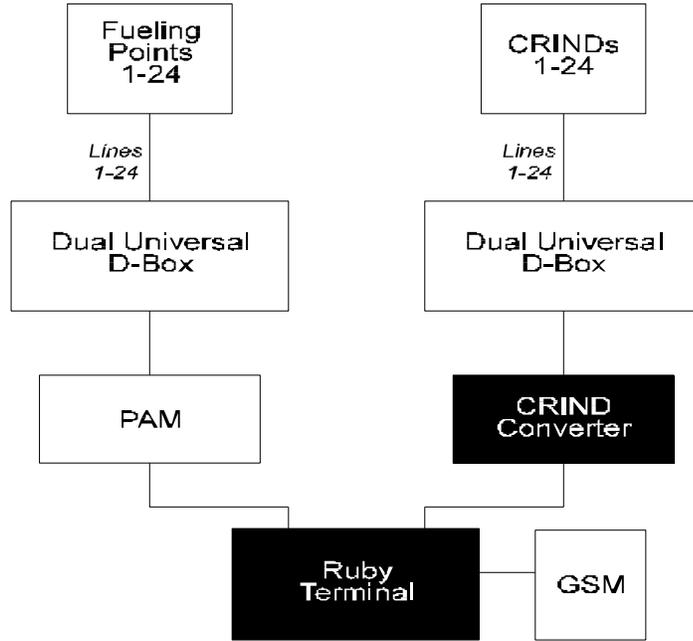
The diagram below illustrates the hardware configuration for 1-32 fueling points with CRIND.
