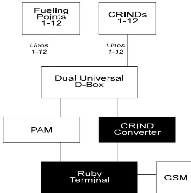
The following diagram illustrates the hardware configuration for 1-24 fueling points with CRIND.
